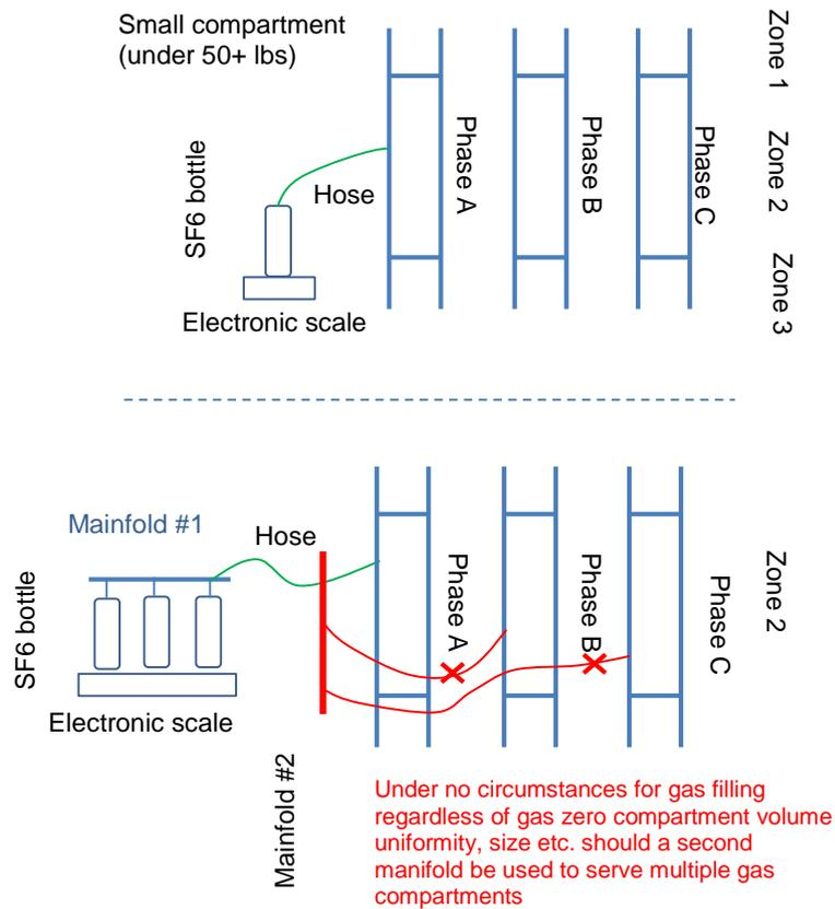
Figure 1. Typical gas weight record and sketch
